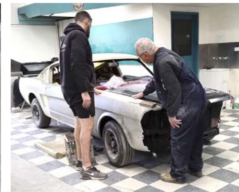
Here you see Gavin and Greg getting the bonnet-to-guard gap into perfect alignment.
