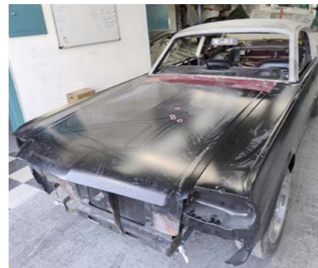
New panels to the doors, guards and bonnet were acquired (painted black in the picture here).
