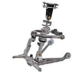
TCP COIL OVER SUSPENSION With Australian Engineering Approval
