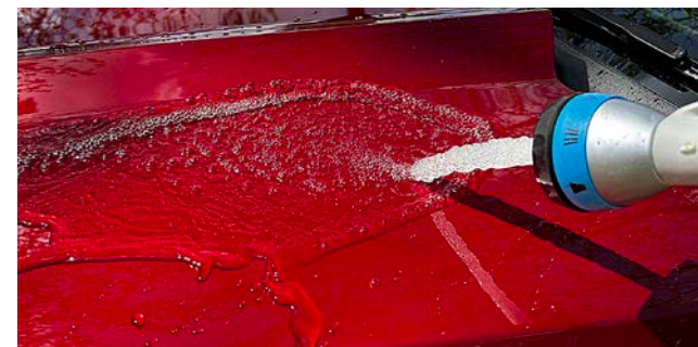
Flood panel with a flow of water for sheeting
