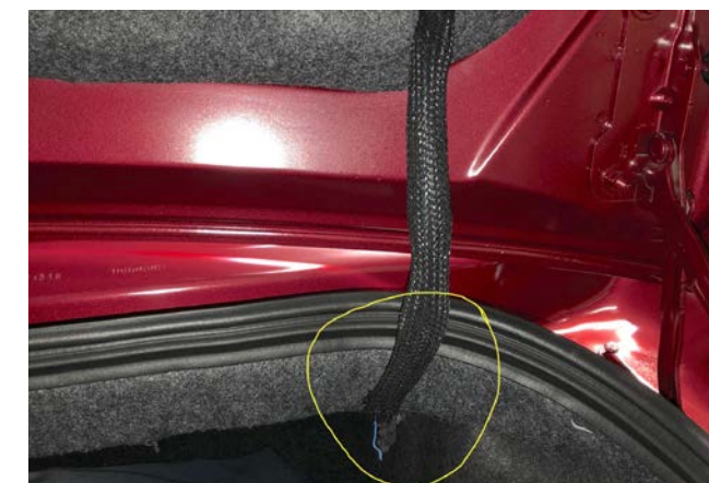
Wiring harness stretched tight when boot was open
