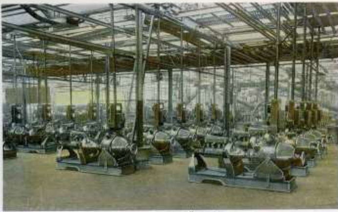
FORD MOTORS RECEIVE A THOROUGH TEST ON THE ELECTRIC "BLOCKS."
