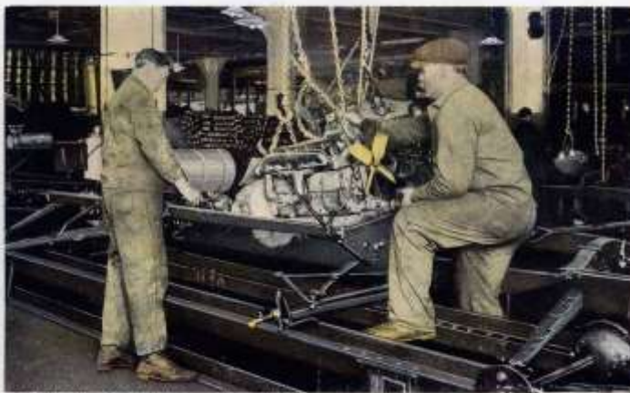
SETTING THE MOTOR, DURING THE FINAL ASSEMBLY.
