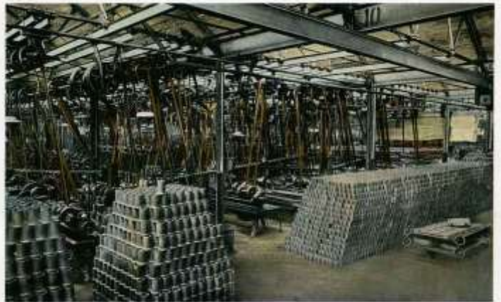
PISTON MACHINING DEPARTMENT. VERITABLE JUNGLE OF BELTS AND SHAFITING.
