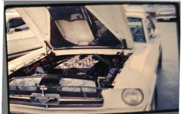
A bonnet scoop was added to improve induction
