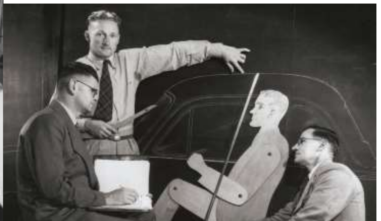
Ford designer Lewis Bandt with two colleagues working with a mannequin to test lumbar support and seating position in 1951. (State Library of Victoria: Wolfgang Sievers)
