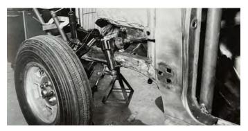
In the development of the funny cars, they received 289 cars from Ford and lengthened chassis and kept modifying, dropping in huge engines in spaces not designed for them. The 427 SOHC and being the focus, but not the only engine used. They developed and used elliptical springs and in order to clear the motors even imported right hand drive steering boxes from Australia (Ford Falcon) and then used these on the outside of the frame!
