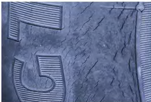
Sidewall cracking due to environmental exposure to oxygen, heat and sunlight.
