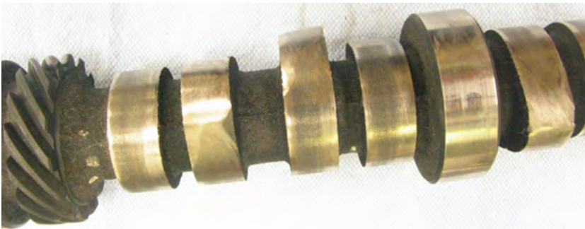
The result of running a flat tappet camshaft using an oil without sufficient ZDDP
